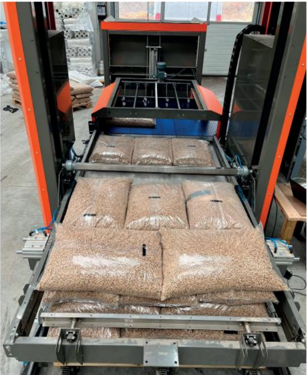
/ 3. A palletizer that automatically places bags on a pallet minimizes the operator's work to collect pallets
